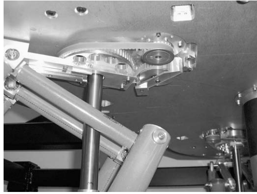
Fig. 10. Actuation system of each leg.
